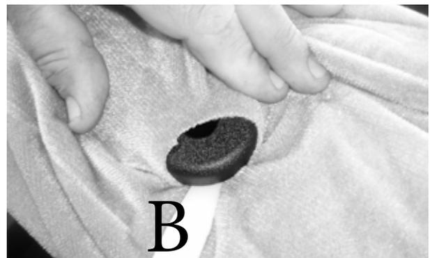
The enclosed installation tool is for your convenience when installing a seat cover. It can be used to tuck the fabric of the seat cover down behind plastic (see picture A), around the headrest housing (see picture B), and other areas as needed.
